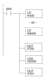
Loads a constant that specifies the number of channels to scan and the data format. The upper byte selects the data format (i.e. 0=BCD, 8=Binary) and the number of channels (set to 4 for the F0–04AD-1).
