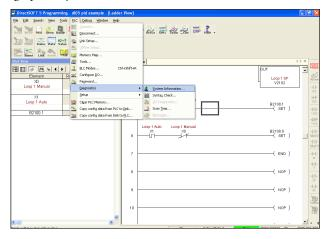
The "CPU Version:" will tell you what firmware revision level is installed in your PLC.
