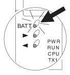
During normal operation, the AC power to the PLC will retain the memory in the Memory Cartridge. If the AC power fails, or is disconnected, a super-capacitor will continue to hold the memory for 4 to 7 days even if the battery is too weak to hold the memory. Only after the capacitor has discharged and the battery has become too weak to retain the memory will program logic and data memory be lost.
