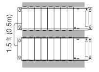
8 slot local CPU base with a 8 slot and 5 slot expansion base
