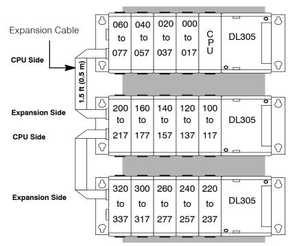
Note: Avoid placing the expansion cable in the same wiring tray as the I/O and power source wiring.
