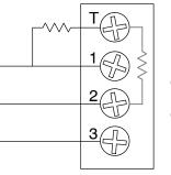
Internal resistor D4-RM - 330 ohm D2-RSS - 150 ohm **Configure Remote** I/O Slaves After configuring the DL350 CPU's Port 2 and wiring it to the remote slave(s), use the following checklist to complete the configuration of the remote slaves. Full instructions for these steps are in the Remote I/O manual.
