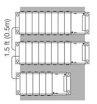
8 slot local CPU base with two 8 slot expansion bases
