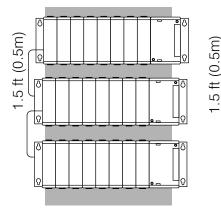
10 slot local CPU base with a 5 slot expansion base
