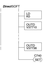
On the last rung in the example program above, we set a special relay contact C740. This particular contact indicates to the CPU the ladder program has finished specifying a remote I/O system. At that moment the CPU begins remote I/O communications. Be sure to include this contact after any Remote I/O setup program.
