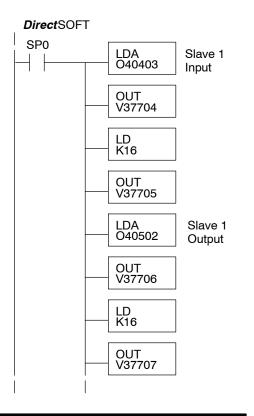
When configuring a Remote I/O channel for fewer than 7 slaves, we must fill the remainder of the table with zeros. This is necessary because the CPU will try to interpret any non-zero number as slave information.
