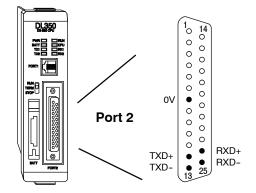
Now we are ready to discuss wiring the DL350 to the remote slaves on the remote base(s). The remote I/O link is a 3-wire, half-duplex type. Since Port 2 of the DL350 CPU is a 5-wire port, we must jumper its transmit and receive lines together as shown below (converts it to 3-wire, half-duplex).
