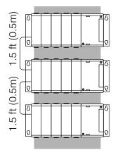
8 slot local CPU base with a 5 slot expansion base
