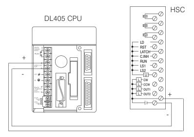
NOTE: When using the internal power supply, make sure your application does not draw more current than the rated 400mA.
