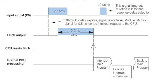
**Multiple Signals from the Same Interrupt Input:** There may be occasions where several interrupt signals are received very close together in time. In the diagram below, the time line reads from left to right. The first signal is latched. It takes 0.5 milliseconds to complete the latching process. If within that time span another signal is sent, the module will ignore the second signal and only recognize the first.
