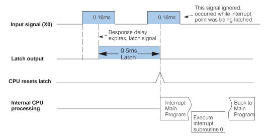
**Simultaneous Signals from** *Different* **Interrupt Inputs:** What happens if the module senses signals simultaneously from several of the interrupt input points? In this case, there is a priority. The highest priority is given to X0, then comes X1, then X2 and so forth down to X7. The diagram below shows two signals being received simultaneously.
