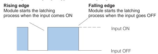
Set the dipswitches to the ON position for rising edge triggering, or set the dipswitches to OFF for falling edge triggering. You will also notice that the points are "paired." That is, one switch sets the triggering for *two* points. For example, If you slide the position 2 switch to the ON position, then *both* inputs 2 and 3 will generate interrupts on the *rising edge*.
