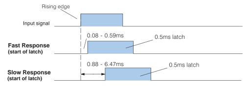
For falling edge triggered signals, the On-to-Off delay is more important. This is because the Interrupt module "waits" for a normally high signal to go low before it recognizes an interrupt. So in this case, the On-to-Off delay filters out any bounce or false signals.
