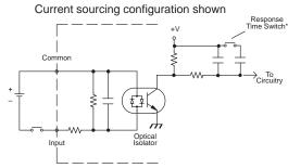
Response delay switch is set with Switch 2, positions 5-8 on rear of the module. This is only for points X0-X3. Points X4-X7 are fixed at the fastest response.
