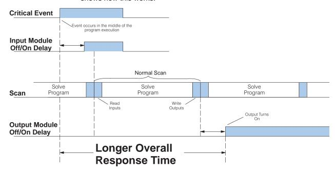
As you can see from the diagram, there can be a delay between the actual occurrence of the event and the CPU processing required to respond to the event. In most applications, the scan happens dozens of times in a second, so the delay is not critical.
