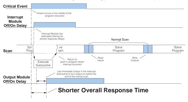
How does the CPU process the interrupts?
