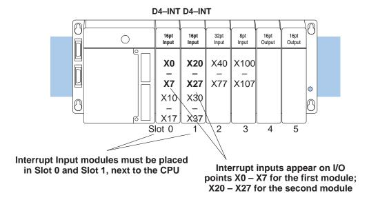
**NOTE:** The D4–440 supports manual I/O configuration. That is, you can manually assign the I/O addresses in any order. If you use manual configuration, make sure you *must* install the Interrupt modules (and use the addressing) as shown above.
