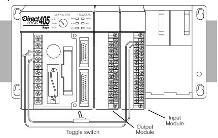
Wire the switches or other field devices prior to applying power to the system to ensure a point is not accidentally turned on during the wiring operation. Wire the input module (X0) to the toggle switch and 24VDC auxiliary power supply on the CPU terminal strip as shown below for the 16ND2 input module. Chapter 2, Installation, Wiring, and Specifications provides a list of I/O wiring guidelines.
