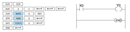
After entering the simple example program turn the key switch from the TERM position to the RUN position and back to TERM. The RUN indicator on the CPU will come on indicating the CPU has entered the run mode. If not repeat Step 10 insuring the program is entered properly or refer to the troubleshooting guide in chapter 9.
