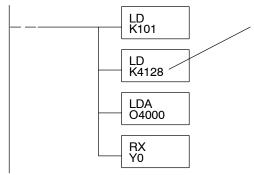
The Maximum constant possible is 4128. This is due to the 128 maximum number of Bytes that the RX/WX instruction can allow. The value of 4 in the most significant position of the word will cause the RX to use function 04 (30001 range).
