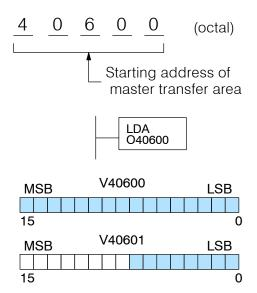
**NOTE:** Since V-memory words are always 16 bits, you may not always use the whole word. For example, if you only specify 3 bytes and you are reading Y outputs from the slave, you will only get 24 bits of data. In this case, only the 8 least significant bits of the last word location will be modified. The remaining 8 bits are not affected.
