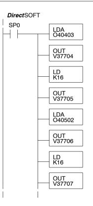
When configuring a Remote I/O channel for fewer than 7 slaves, we must fill the remainder of the table with zeros. This is necessary because the CPU will try to interpret any non-zero number as slave information.
