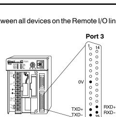
**Configure Remote** I/O Slaves After configuring the DL450 CPU's Port 3 and wiring it to the remote slave(s), use the following checklist to complete the configuration of the remote slaves. Full instructions for these steps are in the Remote I/O manual.
