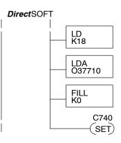
On the last rung in the example program above, we set a special relay contact C740. This particular contact indicates to the CPU that the ladder program has just finished specifying a remote I/O system. At that moment the CPU begins remote I/O communications. Be sure to include this contact after any Remote I/O setup program.
