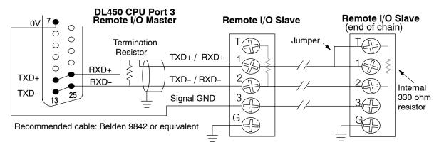
The twisted/shielded pair connects to the DL450 Port 3 as shown. Be sure to connect the cable shield wire to the signal ground connection. A termination resistor must be added externally to the CPU, as close as possible to the connector pins. Its purpose is to minimize electrical reflections that occur over long cables. Be sure to add the jumper at the last slave to connect the required internal termination resistor.
