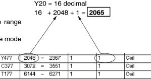
Example 3: T10 Current Value 484 Mode Find the MODBUS address to obtain the current value from Timer T10.
