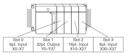
Both the Handheld Programmer and *Direct*SOFT provide AUX functions that allow you to automatically configure the I/O. For example, with the Handheld Programmer AUX 46 executes an automatic configuration, which allows the CPU to examine the installed modules and determine the I/O configuration and addressing. With DirectSOFT, the PLC Configure I/O menu option would be used.
