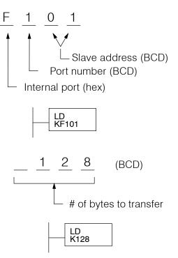
The number of bytes specified also depends on the type of data you want to obtain. For example, the DL405 Input points can be accessed by V-memory locations or as X input locations. However, if you only want X0 – X27, you'll have to use the X input data type because the V-memory locations can only be accessed in 2-byte increments. The following table shows the byte ranges for the various types of **Direct**LOGIC<sup>TM</sup> products.
