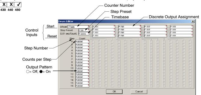
The Timed Drum features 16 steps and 16 outputs. Step transitions occur only on a timed basis, specified in counts per step. Unused steps must be programmed with "counts per step" = 0 (this is the default entry). The discrete output points may be individually assigned as X, Y, or C types, or may be left unused. The output pattern may be edited graphically with **Direct**SOFT.
