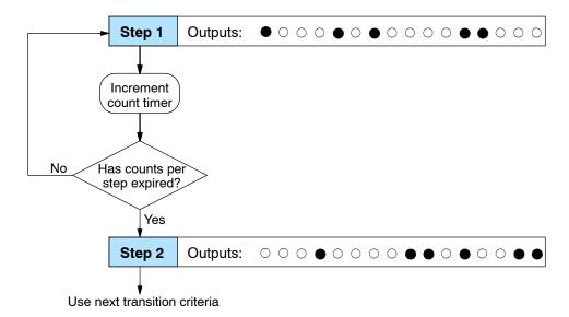
The drum remains in Step 1 for a specific duration (user-programmable). The timebase of the timer is programmable, from 0.01 seconds to 99.99 seconds. This establishes the resolution, or the duration of each "tick of the clock". Each step uses the same timebase, but has its own unique counts per step, which you program. The drum spends a specific amount of time in each step, given by the formula:
