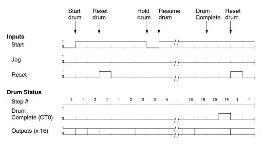
When the drum completes the last step (Step 16 in this example), the Drum Complete bit (CT0) turns on, and the step number remains at 16. When the Reset input turns on, it turns off the Drum Complete bit (CT0), and forces the drum to enter the preset step.
