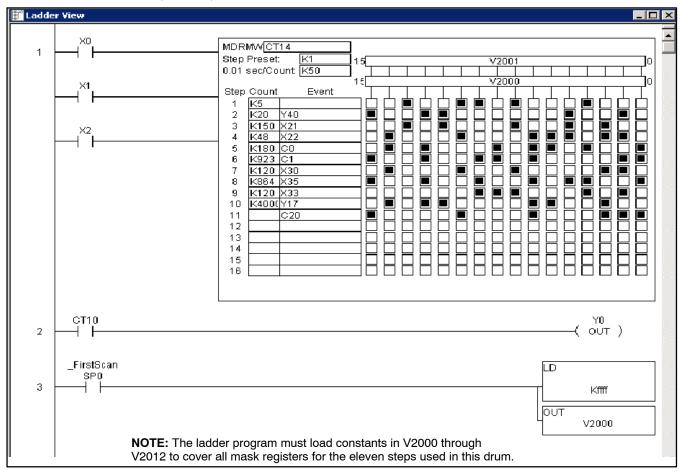
Drum Instruction Programming The handheld programmer can also enter or edit drum instructions. The diagram below lists the keystrokes for entering the drum example on the previous page.
