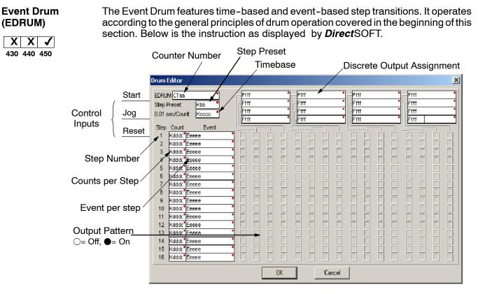
The Event Drum features 16 steps and 16 outputs. Step transitions occur on timed and/or event basis. The jog input also advances the step on each off-to-on transition. Time is specified in counts per step, and events are specified as discrete contacts. Unused steps and events must be left blank. The discrete output points may be individually asssigned.
