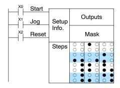
The timing diagram below shows an arbitrary timer drum input sequence and how the drum responds. As the CPU enters run mode it initializes the step number to the preset step number (typically is Step 1). When the Start input goes high the drum begins running, looking for an event and/or running the count timer (depending on the drum type and setup).
