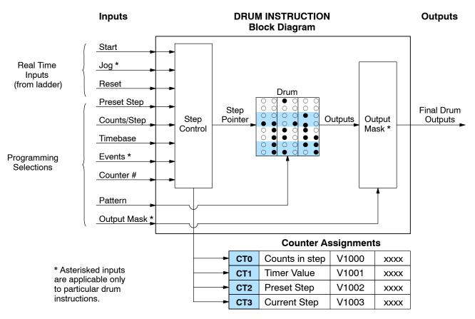
The drum instruction accepts several inputs for step control, the main control of the drum. The inputs and their functions are:
