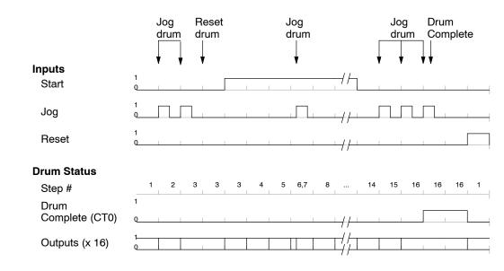
Self-Resetting Applications often require drums that Drum automatically start over thev once complete a cycle. This is easilv accomplished, using the drum complete bit. In the figure to the right, the drum instruction setup is for CT0, so we logically OR the drum complete bit (CT0) with the Reset input. When the last step is done. the drum turns on CT0 which resets itself to the preset step, also resetting CT0. Contact X1 still works as a manual reset.
