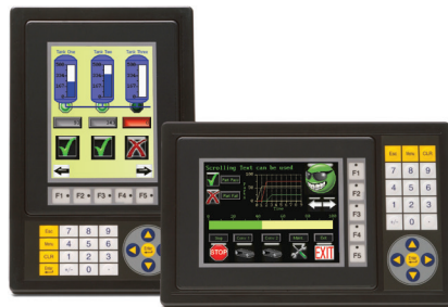
C-more 6" Color Micro-Graphic Panels Installed in Landscape and Portrait Keypad Bezels
