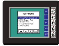
Use the UP [F3] and DWN [F4] function keys to scroll through the list of tests. The BAK [F1] function key will return you to the previous screen. Use the ENT [F5] function key to make your selection once you have the test highlighted.
