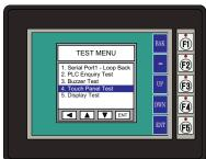
With Touch Panel Test highlighted, press ENT [F5] to bring up the screen shown to the right. Touch any area of the screen to visualize the active area of the touch screen. If the touch panel area is working properly, the screen will blacken at the area touched. Use this test to identify any area that is not responding properly. Press any key [F1 to F5] to return to the Test Menu.
