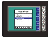
Pressing ENT [F5] with Extensions highlighted will show if an optional keypad bezel is installed on the panel. The example here shows the EA-MG6-BZ2.
