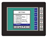
With Rotation highlighted, press ENT [F5] to show the current orientation. Press UP [F3] and DWN [F4] to toggle between the portrait (vertical) and landscape (horizontal) orientation. Use the APL [F5] function button to apply the selection.
