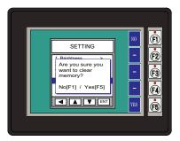
Factory default values can also be reset by pressing F2 and F4 while cycling power to the panel. The Factory Default values are:
