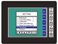
The Hourglass selection listed under the Setting menu can be used to either disable the display of the hourglass icon or set the amount of delay time (0 ms to 1000 ms) desired before it is displayed.
