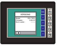
**NOTE**: Software and Firmware Version 3.0 or later is required with model EA1-T4CL. Version 2.5 or later is required with model EA1-T6CL. Available for free download at **www.automationdirect.com**.
