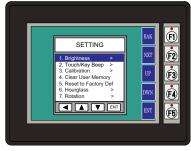
With **Brightness** highlighted, press ENT [F5] to bring up the screen showing the current value. The default is 10. The contrast can be adjusted between 1 and 16, with 1 being the least contrast and 16 being the greatest.
