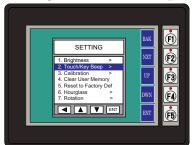
With Touch/Key Beep highlighted, press ENT [F5] to show the current value for the internal beeper. The default is ON. The UP [F3] and DWN [F4] function keys can be used to toggle between the ON and OFF state for the beeper (enable or disable). Use the APL [F5] function key to apply the selection.
