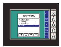
Pressing ENT [F5] with Exit highlighted will allow the used to decided whether to Exit or not Exit the System Setup Screens. See page 5-18.
