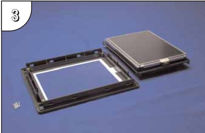
3 Place the new bezel facing down on the lint-free soft surface along with main electronics and four screws.
