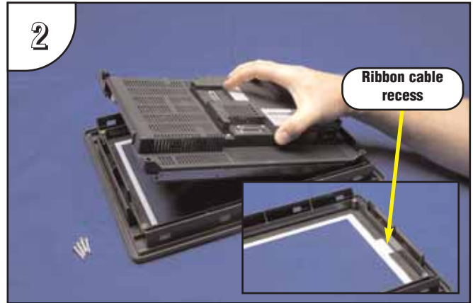
2 Lift the touch panel's main electronics housing from the front bezel. Set the four screws to the side and discard the original bezel. Observe the ribbon cable recess on the front bezel (see detail) for use in re-assembling the panel.
