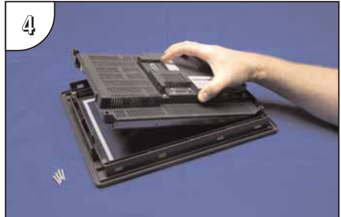
4 Position the touch panel's main electronics housing into the new bezel so that the flat ribbon cable on the housing matches up with the recess in the front bezel. Insert the four screws and tighten to a maximum of 70 oz-in [0.5 Nm].
