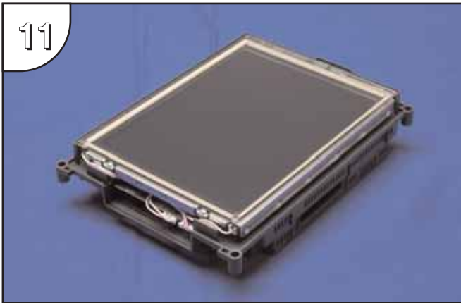
Gently position each backlight bulb's wires back into their respective wire guides to help clear any obstructions when inserting the panel's main electronics housing back into the front bezel. Position any excess wire length in between the printed circuit board and the LCD to prevent it from becoming pinched between the housing and bezel.
