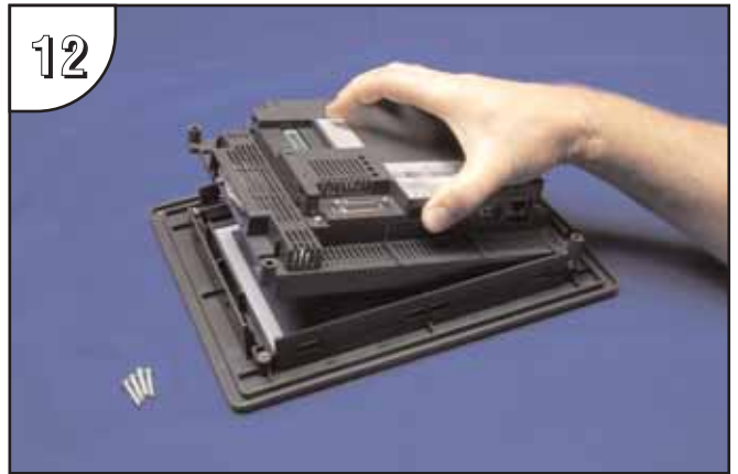
Position the touch panel's main electronics housing into the front bezel so that the flat ribbon cable on the housing matches up with the recess in the front bezel. Insert the four screws and tighten to a maximum of 70 oz-in [0.5 Nm].
