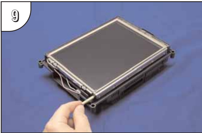
Position the replacement bulb so that the opening in its three-sided gold colored reflector faces toward the LCD touch screen. Using gentle pressure, slide the bulb into the guide until the retaining clip locks.
