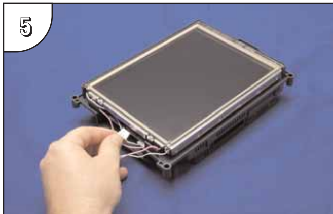
5 Unplug the backlight bulb's power cable connector from the circuit board connector. Again, do this for both the upper and lower backlight bulbs.
