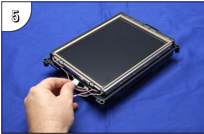
5 Unplug the backlight bulb's power cable connector from the circuit board connector. Again, do this for both the upper and lower backlight bulbs.
