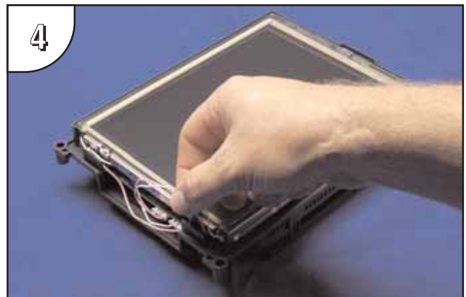
4 Carefully lift the bulb's wires out of the wire guides so they are free from obstructions. Do this for both the upper and lower backlight bulbs.
