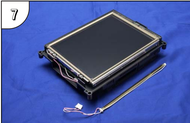
7 This photo shows the backlight bulb completely removed from its guide in the panel's main electronics housing. (Only one bulb shown.)
