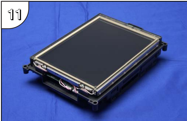
11 Gently position each backlight bulb's wires back into the wire guides. Position any excess wire length in between the printed circuit board and the LCD to prevent it from becoming pinched between the housing and bezel.
