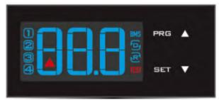
The display shows the temperature in the range of  $-50^{\circ}$ C to  $+150^{\circ}$ C ( $-58^{\circ}$ F to  $+302^{\circ}$ F). The temperature is displayed with resolution of tenths between  $-19.9^{\circ}$ C and  $+99.9^{\circ}$ C ( $-3.8^{\circ}$ F to  $+211.8^{\circ}$ F). During programming, it shows the codes and values of the parameters. The display also shows icons according to occurring events.
