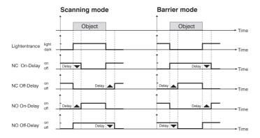
fig. 4 On-Delay and Off-Delay
