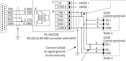
120Ω Termination Resistor at both ends of network
