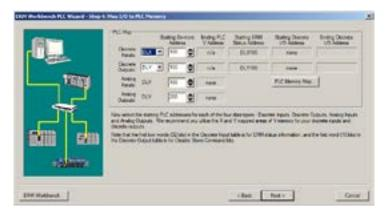
The following window displays how the slave I/O will be mapped into the PLC memory. The network I/O modules and I/O points are listed by slave and slot number. This configuration is written to the ERM by clicking on the "Write to ERM" button. If any advanced configuration needs to be done, click on the ERM Workbench button. The modified configuration can then be downloaded from the ERM Workbench utility to the ERM module.
