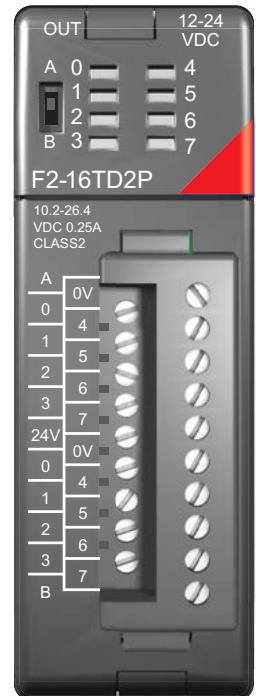
When the A/B switch is in the A position, the LEDs display the output status of the module's first 8 output points. Position B displays the output status of the module's second group of 8 output points.
