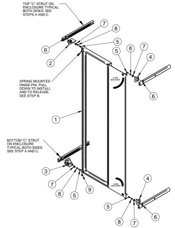
NOTE: MOUNTING HOLES IN THE SIDES OF THE BRACKETS USED IN ILLUSTRATION ARE FOR C2 AND C3 SERIES. USE THE OTHER MOUNTING HOLES IN SIDES OF BRACKETS FOR THE IME AND 1418FS SERIES.
