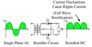
Form factor is the ratio of I<sub>rms</sub> to I<sub>dc</sub> and indicates how close the driving voltage is to pure DC. The form factor for a DC battery is 1.0. The higher the form factor is above 1.0, the more it deviates from pure DC. The Form Factor Table shows examples of commonly used voltages.
