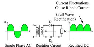
Form factor is the ratio of  $I_{rms}$  to  $I_{dc}$  and indicates how close the driving voltage is to pure DC. The form factor for a DC battery is 1.0. The higher the form factor is above 1.0, the more it deviates from pure DC. The Form Factor Table shows examples of commonly used voltages.
