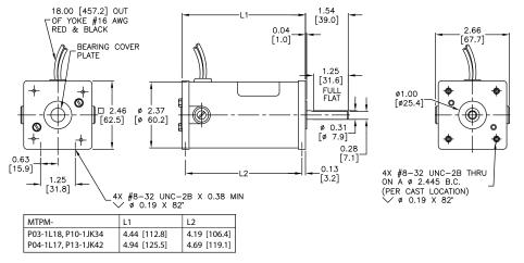
SMALL-FRAME TENV DC MOTORS WITH 0.50-INCH SHAFT DIAMETER - DIMENSIONS
