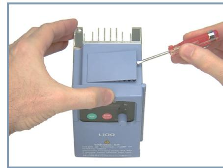
The top housing cover is held in place by four locking tabs. To remove the cover, squeeze two corners together and push a small screwdriver under one side as shown, while pulling upward. Hold the screwdriver at the angle shown, and DO NOT push the screwdriver or any object through ventilation openings and into the inverter.
