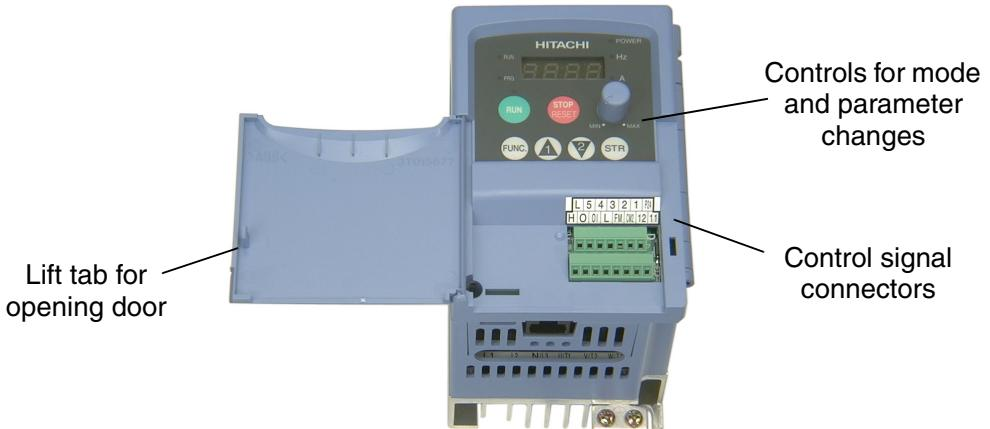
Locate the label sheet that came with the manual. This is a good moment to apply the self-sticking labels as shown below. Adhere the larger label for monitor codes and basic functions to the rear of the half-door panel. Then adhere the remaining trip code label to the area beside the connectors. Be careful not to cover the screw access on models like the one shown.
