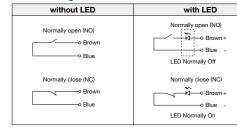
When using the switches with LED option, limit the current below 10mA
