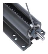
4) Using finger grip, or a 12mm open end wrench, unscrew and remove the lock nut from the lead screw. Hold the carriage steady while turning the nut.
