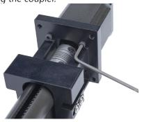
3) Loosen the lock nut set screw at the idler end using a 1.5 mm hex key. Do not remove the set screw completely. Just loosen the set screw 1 or 2 complete turns.
