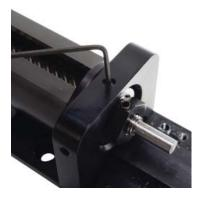
33) Install the new coupler onto the lead screw using a 2mm hex key.
