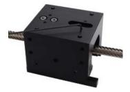
With a 1/16-in hex key, loosen the two side adjusting screws. Loosen one full turn each. Repeat for the other two side adjusting screws on the opposite side.
