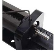
4) Loosen the lock nut set screw using a 1.5mm hex key. Do not remove the set screw completely. Just loosen the set screw 1 or 2 complete turns.
