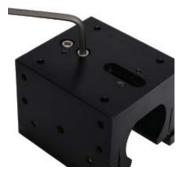
10) Clean all components and remove any debris or accumulated contaminants. Inspect and clean the carriage block, drive screw, and slide tube. All anodized aluminum parts can be cleaned with alcohol or acetone. Avoid contact of cleaning fluid on the slide bushing liners and lead screw drive nut.
