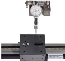
If you need to make adjustments at this point, remember that slight adjustments to the top sliding bushing fasteners have a big impact on the feel and assembly height. Side to side rock is inherent in the round shaft design but is less pronounced when completely assembled.
