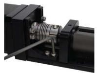
3) Loosen the set screw holding the sensor bracket with a 0.050-in hex key and remove the bracket, and remove the bracket on the opposite end of the actuator.
