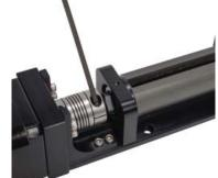
2) Loosen the 4 mounting fasteners at the motor base using a 3/32-in hex key. Remove the motor assembly including the coupler.
