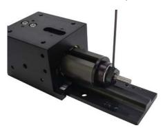
5) Using finger grip, or a 1/2-in open end wrench, unscrew and remove the lock nut from the lead screw. Hold the carriage steady while turning the nut. Repeat the lock nut removal on the opposite end of the actuator.
