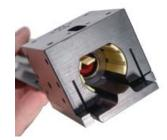
22) Insert the second small slide bushing into the top of the carriage and snap into place.
