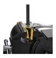
14) Remove the flange mount bearing support unit from the fixed end plate. Use a punch tool such as a large socket and gently tap the bearing from the housing. If necessary, disassemble the housing from the linear rods and use a bench arbor press to remove the bearing. Discard the flanged bearing support unit.
