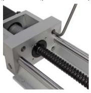
32) Tighten the drive coupler collar lock using a 2.5mm hex key to clamp onto the ball screw.
