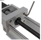
4) Loosen the two set screws on the end support bearing locking nut using a 1.5mm hex key.
