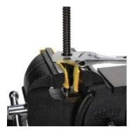
23) The flanged bearing unit is packaged with two spacer sleeves. Install one new spacer sleeve onto the machined and threaded end of the ball screw.
