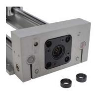
13) Remove the nut block from the ball nut. Move the nut to the end of the ball screw, but do not remove it all the way or the ball bearings may fall out of the nut. Gently clamp the ball nut in a vice with soft jaws. Use a 1.25" open-end wrench, or an adjustable wrench, to loosen the nut block. Discard the used ball nut and ball screw.
