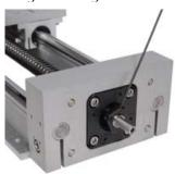
5) Use a 16mm open end wrench to loosen the bearing locking nut. To prevent turning of the ball screw, hold the carriage or the ball screw by hand during loosening. Unscrew, remove, and discard the locking nut.
