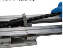
12) Remove the spacer sleeves from the flange bearing inner and outer. The inner sleeve may come apart and be on the ball screw. Discard the two spacer sleeves.
