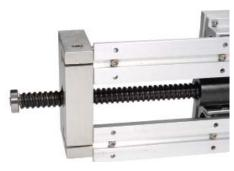
26) Insert the machined and threaded end of the ball screw through the flange mounted bearing support unit. Also ensure that the simple end bearing is seated into the simple end plate.
