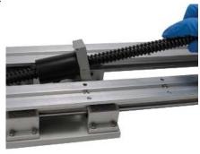
25) Install the simple end radial bearing onto the machined end of the ball screw.
