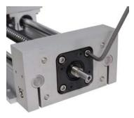
7) Remove the two mounting screws from the top side of the carriage to release the drive screw nut block using a 5/32" hex key.
