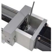
33) Install the retaining ring onto the ball screw at the simple end plate bearing. Use a pair of snap ring pliers to install into the groove.
