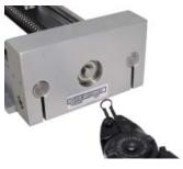
2) Loosen the drive coupler collar lock with a 2.5mm hex key on the coupler screw closest to the ball screw. The coupler can stay attached to the motor and motor mount.
