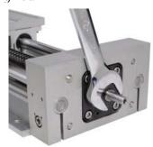
6) Remove the four fixed bearing mounting screws from the bearing flange using a 9/64" hex key.
