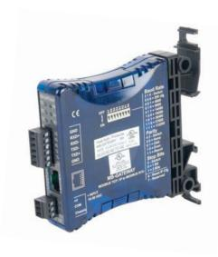
AutomationDirect's MB-GATEWAY is a single port Modbus Gateway module that converts Modbus TCP to Modbus RTU. It supports up to 12 simultaneous Modbus TCP Client (master) Ethernet connections, and up to 128 RTU Server (slave) Serial connections. MB-GATEWAY requires 10VDC to 36VDC from an external power supply. Each module has one RJ45 10/100 Mbps Ethernet port and one RS-422/485 2 or 4 wire Serial Port. It supports NetEdit (Ver 3.8 and later) or Web Browser based configuration tools.
