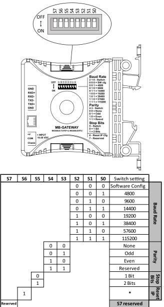
\* Setting S6 to on will, on power cycle, set the IP address, subnet mask and gateway address in the MB-GATEWAY to 0.0.0.0
