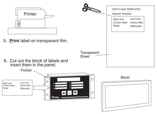
Remove the bezel from the module by unsnapping the four plastic tabs which hold the bezel to the module frame. Locate the pocket, and carefully slide the labels into place. Re-attach the bezel by snapping the bezel onto the case.
