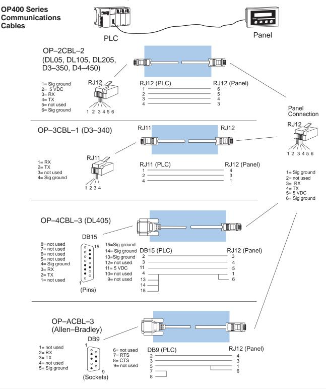
The drawings on this page are for cables which **are not** supplied by **Automationdirect.com**. Use the drawings to make your own cable. We recommend using a 22 AWG or larger shielded cable.
