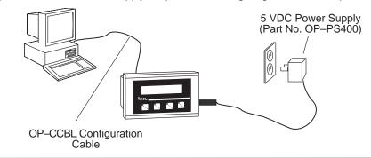
Operation Using a D3–340, D3–350, D3–330 w/DCU, Bottom Port of DL405 or Allen-Bradley CPU: 5 VDC Power Supply Required
