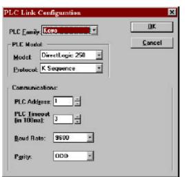
You also have several ports which can be used to connect your communications cable. Some of these ports have fixed PLC address assignments, and some *do not*. The ports which allow configuring the PLC addresses can be set to a unique address, ranging from 1 through 90. **Refer to your User Manual for specific information on the ports of your PLC**.
