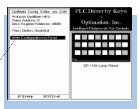
NOTE: Remember that you must have the DIP switch on the rear of the OP-panel set to address 31 in order for the downloading of your configuration to take place.
