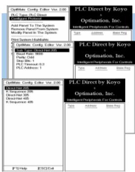
Step 6B Set the Baud Rate, Parity and Stop Bits
