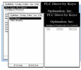
Step 6A Select Configure Protocol and the PLC Subtype Select **Configure Protocol**. Here we are selecting the communications protocol that will be used between the PLC and the OP-9001.
