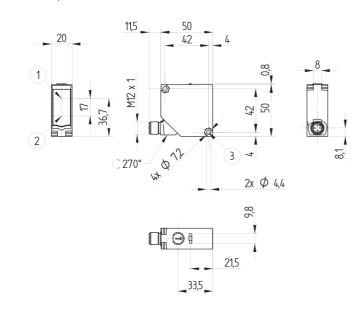
① = Emitter diode ② = Receiving diode Screw M4 = 0,5 Nm Potentiometer = 40 Nmm Dimensions specified in mm (1 mm = 0,03937 Inch)
