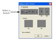
The **Display Switch** window will close and the **Waterworks** screen will appear again. The switch just selected should now be displayed on the **Waterworks** screen. The switch position is adjustable and it can be dragged and placed anywhere on the **Waterworks** screen.
