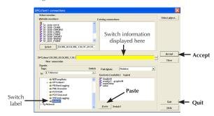
Once the switch reference text is shown on the address line, click on the **Accept** button to accept the output point and switch selections. Clicking on **Quit** will close the **OPC Client Connections** window.
