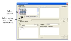
From the top left list, click on the device with the slot number and output point you want to use for your sample project. The output point will be highlighted. Now click on the **Select** button. The information for the output point will be displayed next to the **Select** button.
