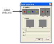
The **Display Logical Signal** window will close and the **Waterworks** screen will be displayed. The indicator just selected should be displayed on the screen. You can click on the indicator and drag it next to the new switch created in the previous steps.
