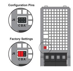
Figure 1 – Configuration Jumpers (Top of Unit)
