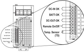
Figure 2 – Signal Connector Pinout (Bottom of Unit)
