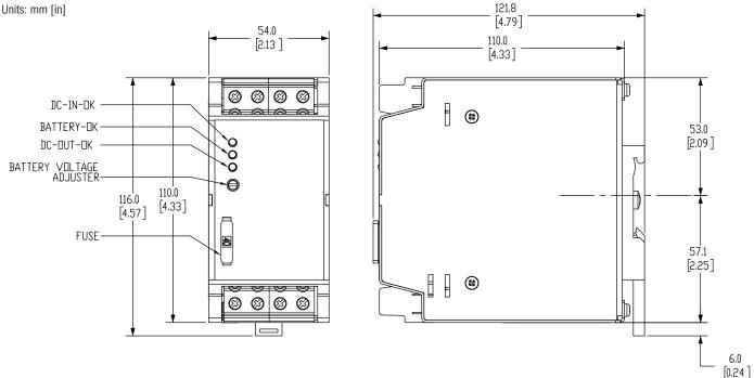
The correct mounting position for optimal cooling performance must be observed: Mount upright on horizontal DIN rail. Do not cover any ventilation holes. Leave a free space of minimum 80mm [3.15 in] above and below the power supply and on each side of the power supply a minimum space of 25mm [0.98 in] which allows air convection.
