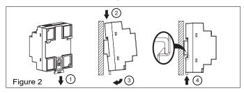
Snap on the DIN rail as shown in Fig. 2:
