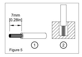
In accordance with EN60950 / UL60950, flexible cables require ferrules.
