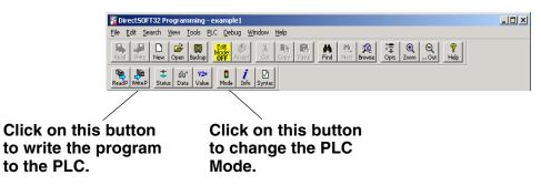
The program has now been written to the PLC. All that needs to be done now is to put the PLC in the RUN mode. Click on the **Mode** button on the online toolbar. This will bring the **PLC Modes** dialog window into view. Click on **Run** then **OK** and the PLC will be in the **RUN Mode**.
