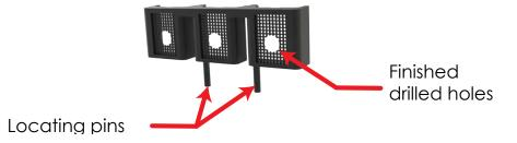
6) When drilling is complete, install the finger guards to the supply and load sides of the SR35 soft starter.
