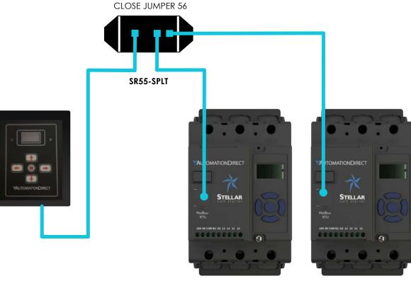
ADDRESS = 1 Enable keypad power on this unit only
