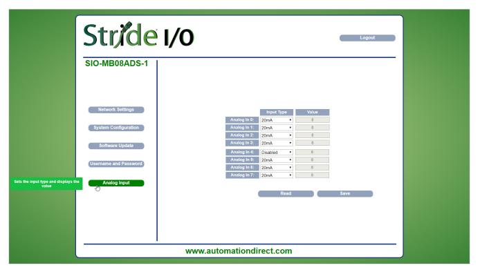
This page displays the values of the analog inputs in the unit of measurement defined by the "Input Type". Each Input can be disabled selecting "Disabled" in the combobox under the column "Input Type".
