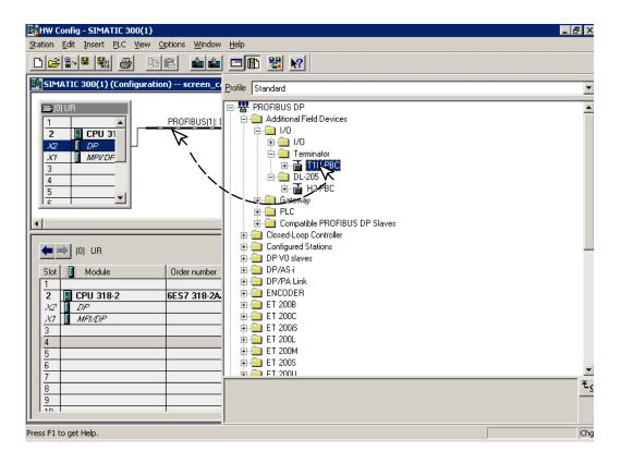
When the mouse button is released at the network node, the **Properties** window will appear so the correct node address can be entered. The transmission baud rate can be changed at this time also. Click **OK** when finished.
