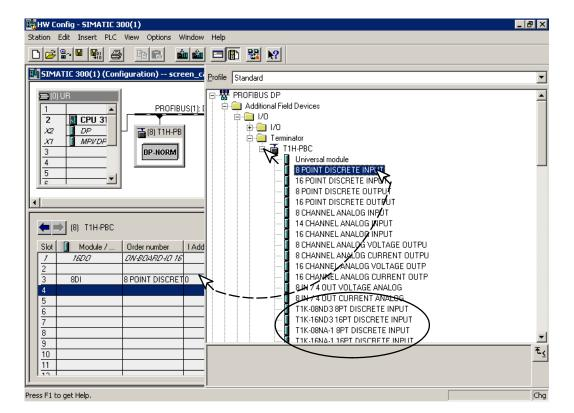
After you have finished configuring the I/O for the T1H–PBC DP Slave, the configuration window will look like the example below.
