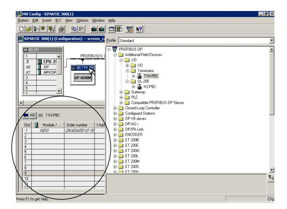
Open the T1H–PBC I/O list by clicking on the + sign next to T1H–PBC. Now you can chose the I/O modules which are installed in your Terminator base. You have the option of selecting the generic I/O or the Terminator I/O part number. The generic name is selected in this example.
