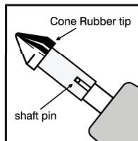
2. Bring cone into contact with the shaft. Apply only enough pressure to avoid slippage.
