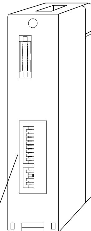
DIP Switches for communications and Protocol Setup
