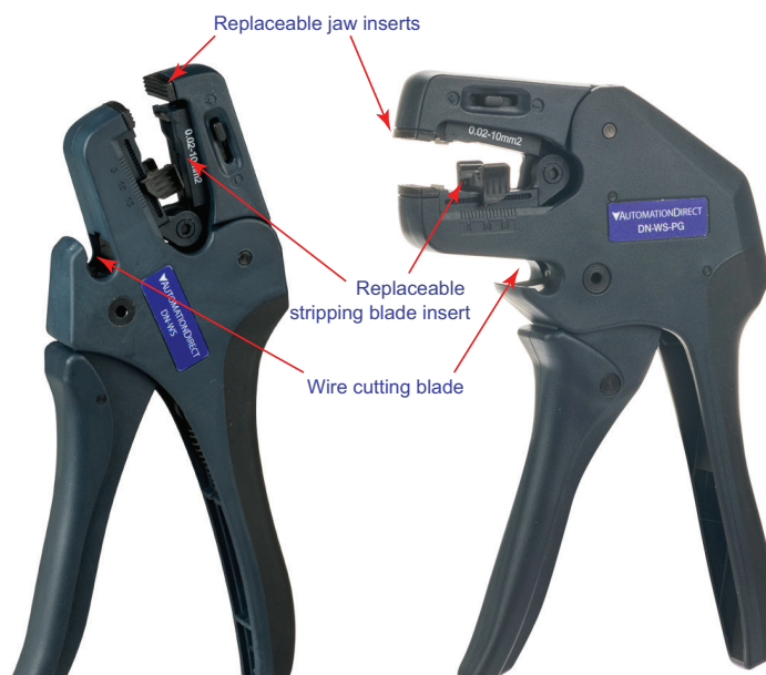
DN-WS Cutting & Stripping Tool
