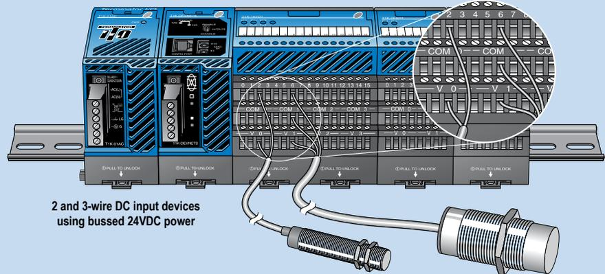
2 and 3-wire DC input devices using bussed 24VDC power
