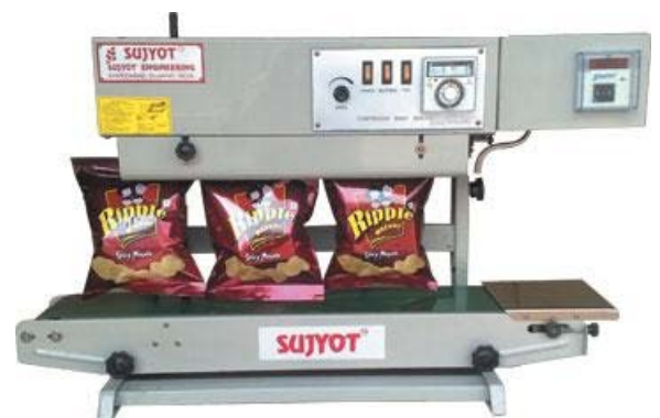
Continuous Sealing Machine with Nitrogen Flushing
