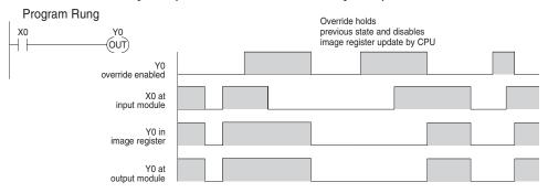
The following diagram shows how you can use a programming device in combination with the bit override to change the status of the point. Remember, bit override only disables CPU changes. You can still use a programming device to force the status of the point. Plus, since bit override maintains the current status, this enables true forcing. The example shown is for an output point, but you can also use the other bit data types.
