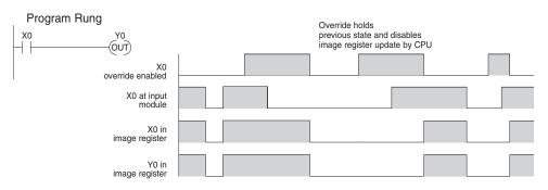
The following diagram shows how the bit override works for an output point. Notice the bit override maintains the output in the current state. If the output is on when the bit override is enabled, then the output stays on. If it is off, then the output stays off.
