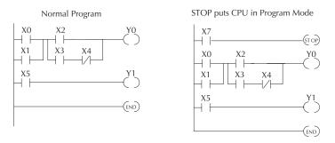
In the example shown above, you could trigger X7 which would execute the STOP instruction. The CPU would enter Program Mode and all outputs would be turned off.
