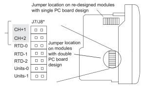
\* Jumper is designated J8 on double PC board models and J7 on single PC board models.
