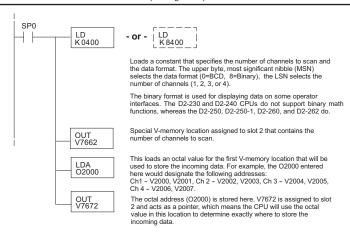
The following tables show the special V-memory locations used by the D2-240, D2-250-1, D2-260 or D2-262 for the CPU base and local expansion base I/O slots. Slot 0 (zero) is the module next to the CPU or D2-CM module. Slot 1 is the module two places from the CPU or D2-CM, and so on. Remember, the CPU only examines the pointer values at these locations after a mode transition. Also, if the D2-230 (multiplexing) method is used, verify that these addresses in the CPU are 0 (zero).
