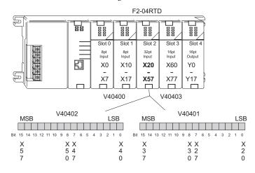
When a D2-230 CPU is used, the input points must start on a V-memory boundary. To use the V-memory references required for a D2-230 CPU, refer to the table below. The first input address assigned to a module must be one of the X inputs shown. The table also shows the V-memory addresses that correspond to these X inputs.
