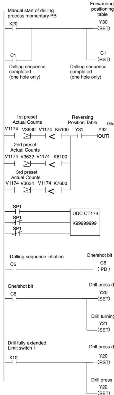
The operator starts the drilling by moving the positioning table forward. A quadrature encoder is transmitting the pulses to the D2-CTRINT module. After 5000 pulses are counted, the positioning table is stopped and the drilling sequence is started. Two more holes are needed in this work piece so the positioning and drilling are repeated twice automatically. (Stop and jog buttons are left out here for simplicity but should be incorporated in your logic.).
