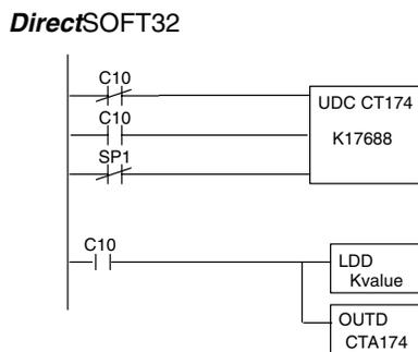
C10 is shown normally closed. When pulses are received at point 00, the current value in CTA174 will increment. When pulses are received at point 01, the current value will decrement. When C10 energizes, CTA174 stops counting and Kvalue is loaded for a new preload value. When an input is received at point 02, the counter will reset.
