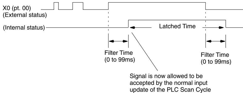
**Note:** If zero is put in V-memory as the filter time. The CPU will treat the configuration as having no filter.
