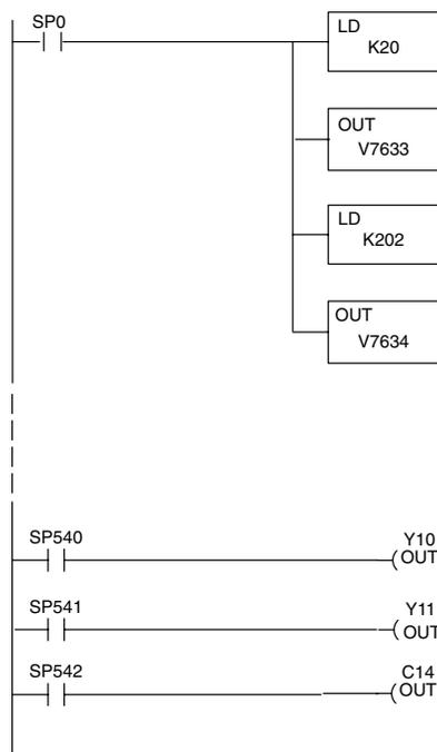
} Equal relays used to trigger outside events. Can be used in the main program and in subroutines.
