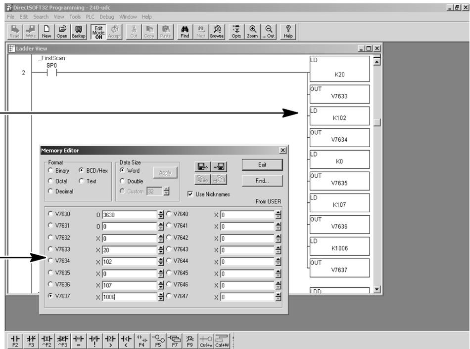
Editing the D2-CTRINT setup at the beginning of the user program is the most efficient method for setting up the counter mode. Should there be a need to change any of the counter setup values after the PLC has been put in the RUN Mode, use the Memory Editor to change the values. These values will only be temporary. They should be put into the program if they are to be used permanently.
