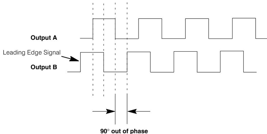
Now Output B is the leading signal, and it will cause the counter to count down. This would indicate to the CPU that the motor shaft is turning *counter-clockwise*.
