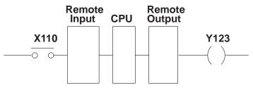
The drawing below shows the details of the CPU and Remote Master interaction .
