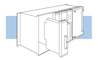
Align module to slots in base and slide in
