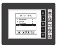
Pressing ENT [F5] with Exit highlighted will allow the used to decided whether to Exit or not Exit the System Setup Screens. See page 5-18.
