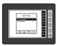
Use the UP [F3] and DWN [F4] function keys to scroll through the list of settings. There are six selections on the first screen and two additional selections on a second screen. You can also use the NXT [F2] function key to go back and forth between the two screens without having to use the up and down keys. The BAK [F1] function key will return you to the previous screen. Use the ENT [F5] function key to make your selection once you have the setting highlighted.
