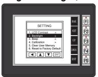
With Backlight highlighted, press ENT [F5] to show the current backlight screen color. For model EA1-S6ML, the default is green. The UP [F3] and DWN [F4] function keys can be used to scroll through the five available backlight colors (green, lime, yellow, amber and red). Use the APL [F5] function key to apply the new color. Shown here are the various backlight colors.
