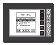
**Serial Port1** - Performs a test to verify the RJ12 serial communications port (Port 1) on the panel is operating correctly. Requires a loop back connector inserted into the port to properly run the test. A wiring diagram for the loop back connector is shown below.
